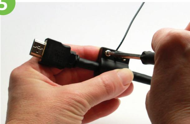
Hold the clamp with your finger, turn it around and tighten it with the provided screws.
