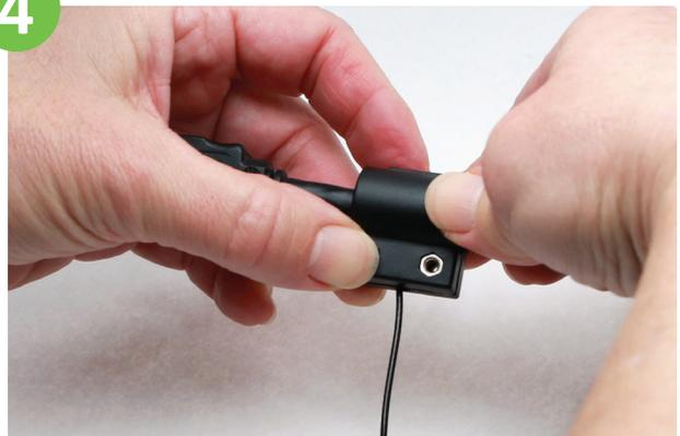
Hold the clamp with your finger, turn it around and tighten it with the screws provided.
