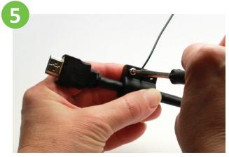
Hold the clamp with your finger, turn it around and tighten it with the provided screws.
