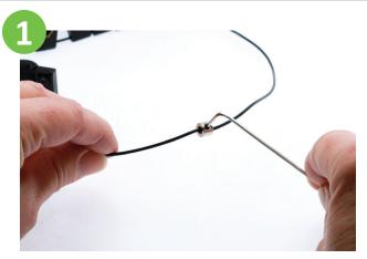
Use the 1.5 mm Hex wrench to screw the black screw of the wire connector halfway up.
