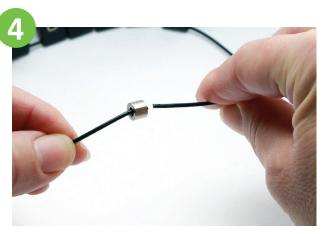
Guide the two wire ends back into the wire connector.
