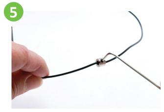
Tighten the black screw of the wire connector with the 1.5mm Hex wrench.
